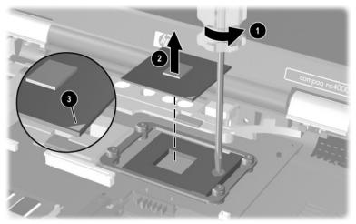
Removing the Processor
